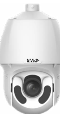
VIS-P2PTZXIR33NH 2 Megapixel IP Plug & Play, Outdoor PTZ, Motorized Auto-Focus, up to 492 IR Range, WDR, Audio Input/ Output, SD Card Slot, 24VAC/PoE+
